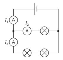
The readings on the ammeters are  $I_1$ ,  $I_2$  and  $I_3$ .
