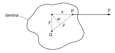
The lamina is free to rotate about point Q.
