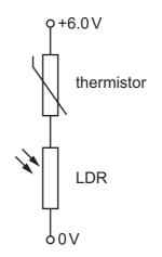
The thermistor has a resistance of  $6000 \Omega$  in a cold room and  $1000 \Omega$  in a warm room. The LDR has a resistance of  $2000 \Omega$  in dim light and  $500 \Omega$  in bright light.
